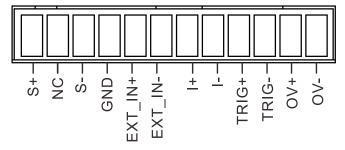
Figure 12 Control Signal Terminal
