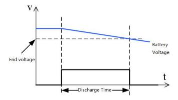
Figure 32 Discharge test curve
