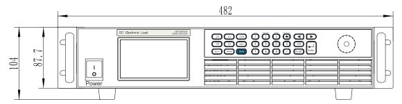
Figure 3 Front Panel Dimension(mm)
