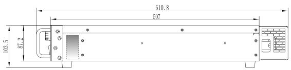
Figure 5 Side Dimension(mm)
