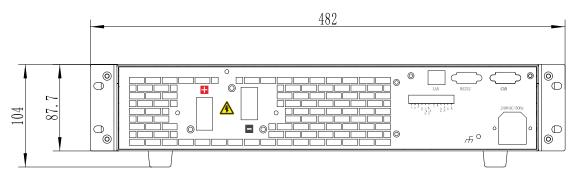
Figure 4 Rear Panel Dimension(mm)
