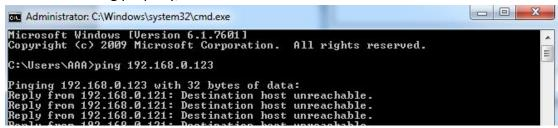
Figure 68 Communication Test
