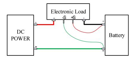
Figure 34 Charge Test Wiring Diagram
